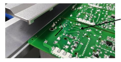
The pins cannot be bent too far, The distance is better than 2mm, to facilitate machine cutting efficiency
